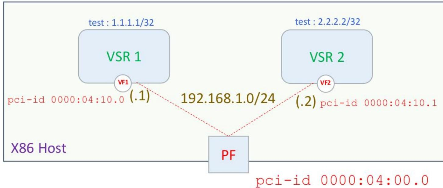
1. An IPsec tunnel is established between the two VSR over the IPv4 network 192.168.1.0/24 which uses the VF to VF communication channel
